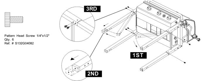
**2 NOTE:** Before attaching the Cart Bottom Shelf to Cart be sure tank hole on the Bottom is located on the right side.
